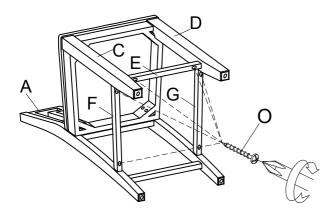
Stand chair up on an even surface and check that it is balanced. If there is a slight wobble, apply downward pressure in the corner where a leg is uneven. Keeping pressure in that corner, tighten all bolts. If balanced, apply downward pressure evenly in the center and tighten all bolts. Do not over-tighten beyond hole depth.
