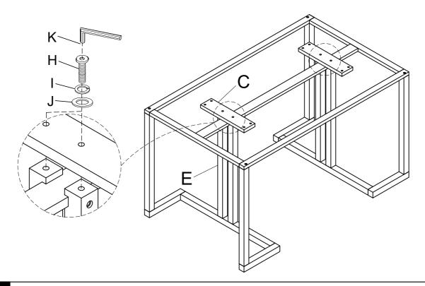
Turn the assembly over. Attach the Middle Post (E) to Foot Frame (F) by Bolt (G), Lock Washer (I) and Flat Washer (J) with Allen Wrench (K) as shown.
