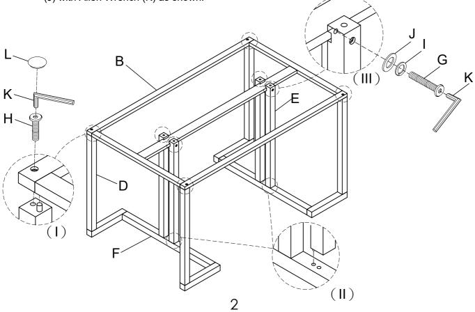
Attach the Joint Panel (C) to Middle Post (E) by Bolt (H), Lock Washer (I) and Flat Washer (J) with Allen Wrench (K) as shown.
