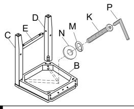
Take the Allen Wrench, and turn the bolts until the legs are secured. DO NOT TIGHTEN COMPLETELY. Stop when you feel you are adding force to tighten the bolt.
