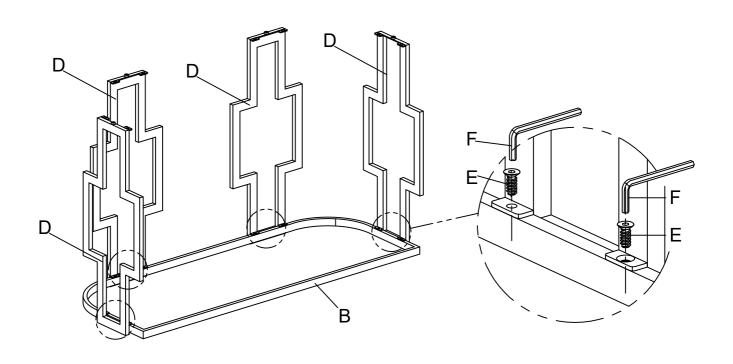
Attach Bottom Frame (C) to the pre-assembled Side Frame (D) using Bolt (E) by Allen Key(F) as below shown.
