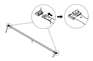
Attach the assembled Slats (I) to the daybed rails, insert the Slat Connector (J) into the correct holes.
