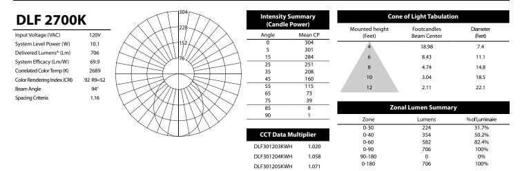
Fixture tested per LM-79-08. Photometric data is of the performance of a representative fixture with round white trim. Results may vary in the field.
