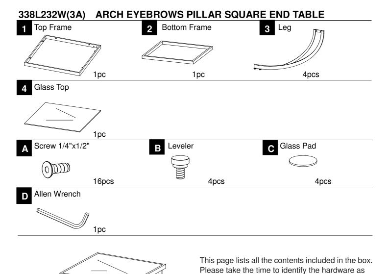
\*\*\* Do not tighten screws & bolts until the entire unit is completely assembled.
