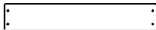
M9 TABLEAU DE SOL - W4L17660 (x10) 5/8 po x 3/8 po x 19 7/8 po (16x86x504)
