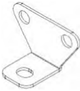
J7 SUPPORT À CHEVRON - A4M03802 (x4) 3 5/8"x2 3/16"x2" (50x55x92)
