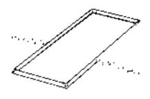
2. Place Flange Kit in ceiling opening and wire each corner to ceiling structure. Pull up tight against ceiling.
