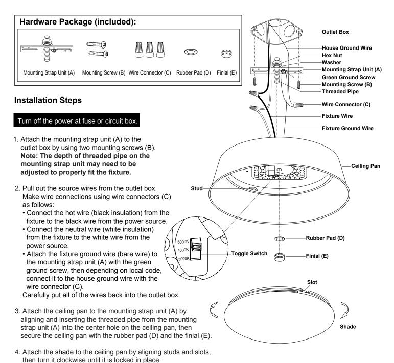
Turn on the power at fuse or circuit box.
