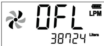
If the flow rate goes out of measurable range, (as in the diagram above), "OFL" will appear on the display screen.
