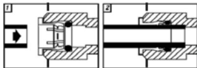
Insert the hose towards the direction where the arrow points to install.
