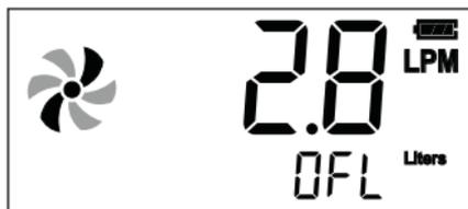
If the cumulated flow rate goes out of measurable range, (as in the diagram above), "OFL" will appear on the bottom of the display screen.
