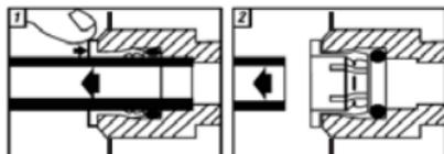
While pressing the grey ring, pull the hose towards the direction where the arrow points to separate the hose.
