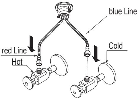
Connect hot and cold waterlines (7) to the angle stops. Tighten with a wrench until snug. Turn on hot and cold angle stops and check for leaks
