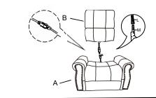
STEP 4: Connect the power and open/close the footrest by pressing the button.
