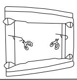
STEP 3: Install the wings by inserting metal bracket on the LSF wing (C) and RSF wing (D) into the metal bracket on the backrest (B). Please make sure the brackets are inserted all the way and secured into position.
