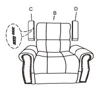
STEP 2:Install the backrest (B) by align and insert the metal bracket on the backrest (B) to the metal bracket of the seat (A). Connect the wire between the backrest (B) with the wire on seat (A). Please make sure the brackets are inserted all the way and secured into position.
