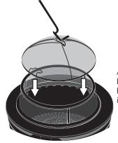
After a Wood Pack or firewood has been added, place the top piece back on with the poker. Ensure that it is securely nested.
