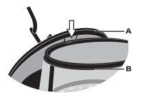
To add an additional Wood Pack or firewood, remove the top piece (A) of the screen with the included poker (see page 6 for assembly), and gently hang on the side of the bottom piece (B).
