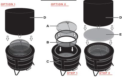
When the Fire Pit is not in use, place the cover (D) (included with the Fire Pit purchase), over to help protect your screen and Fire Pit from the elements.
