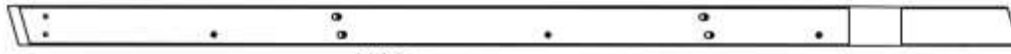
H01 | SOLIVE DE TOIT - W4L16295 (1) | 1 po x 3 3/8 po x 88 3/16 po (24 x 86 x 2 240)
