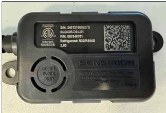
FIGURE 32. Example of Clear, Unobstructed Sensor Inlet
