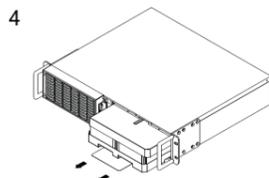
4. Pull out the old battery pack and replace new one. Reassemble the retaining screws, covers, black and red cable, and front panel in the reverse sequence of the above steps. Recharge the unit for 12 hours to ensure maximum UPS battery runtime.
