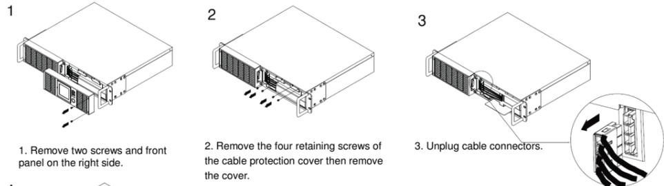
1. Remove two screws and front panel on the right side.
