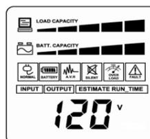
**INPUT voltage meter:** This meter measures the AC voltage that the UPS system is receiving from the utility wall outlet. The INPUT voltage readout can be used as a diagnostic tool to identify poor-quality input power. The AVR in this UPS continuously conditions the power to a stable 110/120V output to connected equipment. In the event of a complete power loss, severe brownout, or over voltage, the UPS relies on its internal battery back up to supply a consistent 110/120V output.
