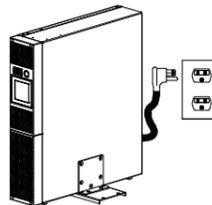
Unplug the unit and turn Power Off when first connecting your computer and peripherals.
