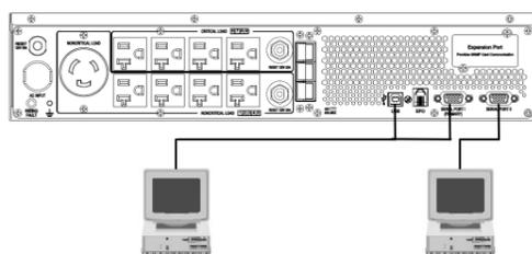
Install PowerPanel® Business Edition software on the primary computer connected to UPS with either a serial cable or USB cable.
