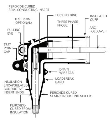
Figure 1. Line illustration of 200 A 35 kV Class elbow.
