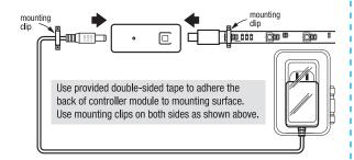
Connect power supply to wall outlet.
