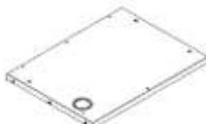
T6 ASSEMBLAGE DE TABLE - A4M05601 (x1) 1 3/8"x23 3/8"x31 7/16" (35x594x798)
