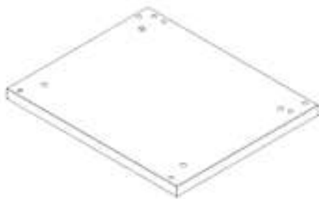
T5 - ARMOIRE PANNEAU R- A4M03069 (x1) 1 1/4"x20"x24 1/8" (32x508x612)
