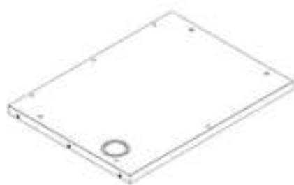
T6 ASSEMBLAGE DE TABLE - A4M05601 (x1) 1 3/8"x23 3/8"x31 7/16" (35x594x798)
