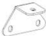
J3 SUPPORT DE CHEVRON - A4M02984 (x5) 2"x2 3/16"x3 5/8" (50x55x92)
