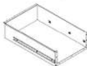
D10 MONTAGE DE TIROIR - A4M03081 (x4) 5 11/16"x14 5/8"x22 1/4" (145x372x565)
