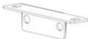
A8 SUPPORT DE TABLE- A4M03149 (x1) 1 15/16"x1 15/16"x7 1/2" (50x50x191)
