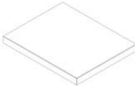
M2 CABINET COUNTERTOP L - A4M05969 (x1) 1 15/16"x20 1/16"x24 13/16" (50x509x630)
