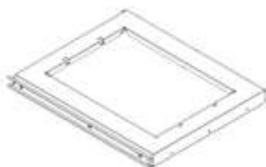
A15 SUPPORT DE POUBELLE- A4M03085 (x1) 1 3/8"x14 11/16"x450.00 (35x373x455)
