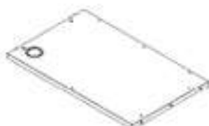
T2 ASSEMBLAGE DE TABLE - A4M03057 (x1) 1 1/4"x23 3/8"x38 3/16" (32x594x970)
