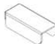
A5 SUPPORT D'ÉTAGÈRE - A4M03141 (x8) 5/8"x7/8"x2 1/16" (16x22x53)
