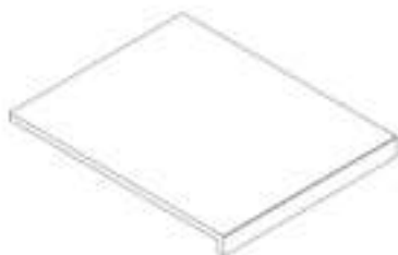
M3 COMPTOIR D'ARMOIRE R - A4M05970 (x1) 1 15/16"x20"x24 13/16" (50x508x630)
