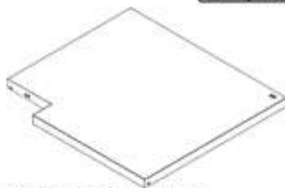
C4 ARMOIRES DE GRIL- A4M03046 (x1) 1 1/4"x23 1/8"x25 7/16" (32x588x646)
