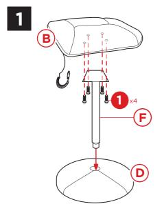
Attach part F ottoman support to bottom of part B ottoman seat with four part 1 screws. Insert the ottoman support and seat into the part D ottoman base.
