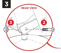
Unfold the chair. Insert two part 2 bolts into the hinges on the back of the chair and secure them with two part 3 nuts.
