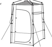
STEP 12: Unfold fly and place it over tent. Attach the hooks on the fly corners to the metal rings on the main upright poles.
