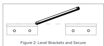
3. Secure the brackets to the wall.
