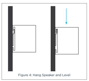
5. If the speaker is at an acceptable height/level, then wire and hang the speaker and attach the grille to complete the installation.
