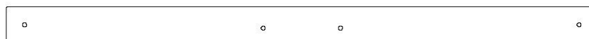
H13 | SUPPORT DE POUTRE DE BALANÇOIRE - W4L06533 (x1) | 1 po x 3 3/8 po x 54 3/8 po (24x86x1380)
