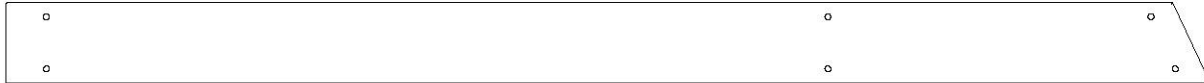
G3 | PLANCHE DE SOL - W4L16878 (x1) | 1 po x 5 1/4 po x 78 1/2 po (24x134x1995)
