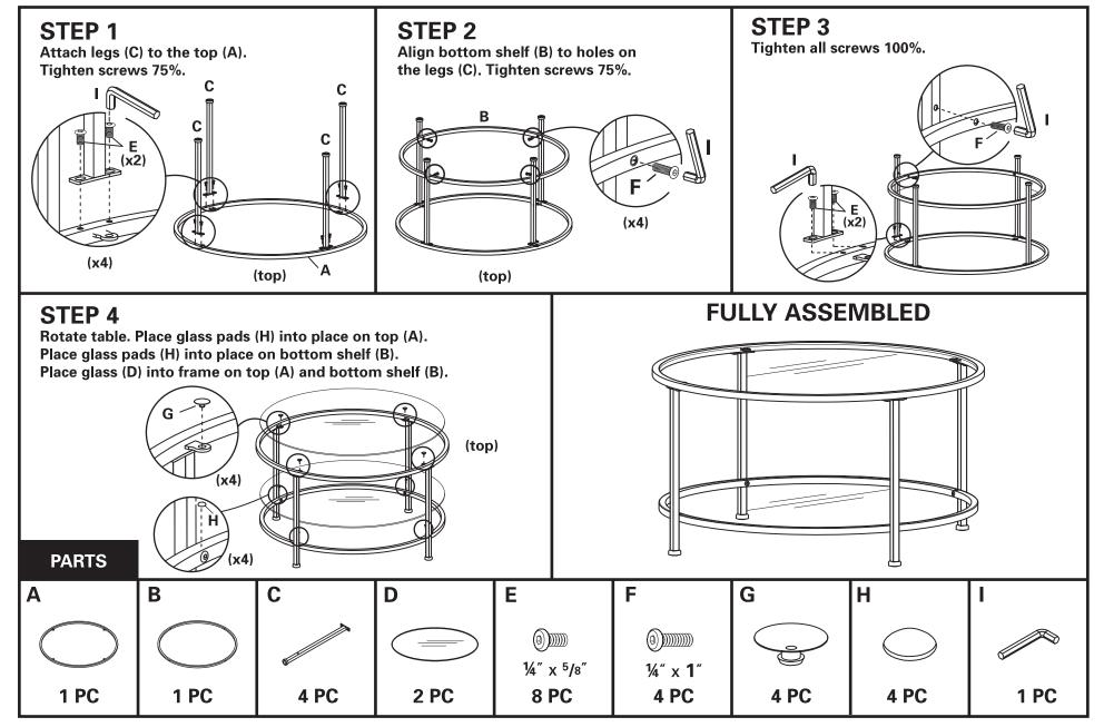
NOTE: DO NOT TIGHTEN SCREWS 100% UNTIL COMPLETELY ASSEMBLED
