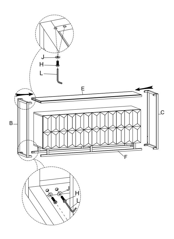
3 Attach Back Support (D) to the back of Top Panel (E), Left Side Frame (B) and Right Side Frame (C), using Bolt (H), Flat Washer (J) by Allen Key (L) as below shown.
