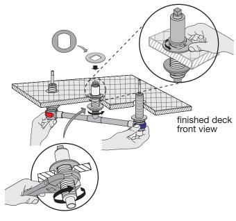
Step 4 Attach supply valves to deck
