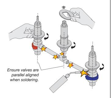
Step 3 Attach spout centerbody to deck
