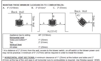
\*\* <u>VERTICAL VENT SECTIONS:</u> A minimum of 1" (25mm) all around the vent pipe on all vertical runs to combustibles is required. Use firestop spacer W500-0097 (not supplied).
