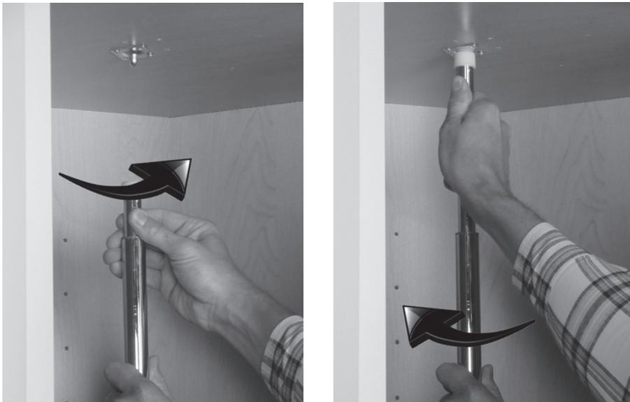
Holding onto the lower pole twist the upper pole counter clockwise to release. Extend pole upwards until it rests firmly against the Top Mounting Support and tighten by turning the pole clockwise.
