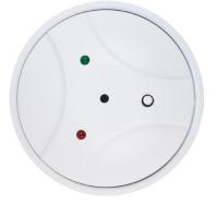
The Glass Break Detector (2GIG-GB1-345) is a fully-supervised, tamperprotected, ceiling- or wall-mounted unit. It communicates with the 2GIG Control Panel using the 345 MHz frequency. The detector provides a 15 ft (4.6 m) maximum detection range, 360° maximum horizontal sensing angle, and dual-stage glass break detection.
