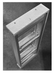
**Face Frame Application:** Measure the overlay of adjoining cabinet stile to determine scribe rail thickness (not included). Rail thickness = Measurement + 1/4". **Frameless Application:** Recommended scribe rail thickness is 1/4".
