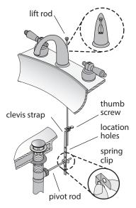
If necessary, select another *location hole* in *clevis strap* and re-adjust *lift rod* where fastened to *clevis strap*.
