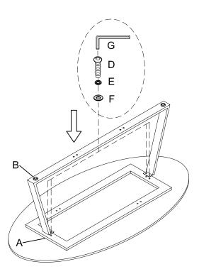
Attach the L Leg (C) to the Table Top (A) and the U Leg (B) using Bolt (D), Spring Washer (E) and Flat Washer (F) with the Allen Key (G).
