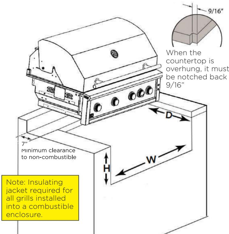
Note: Insulating jacket required for all grills installed into a combustible enclosure.
