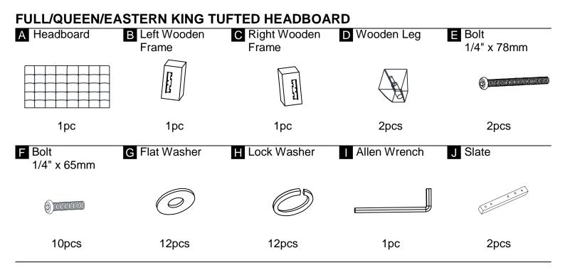
This page lists all the contents included in the box. Please take the time to identify the hardware as well as the individual components to this product. As you unpack and prepare for assembly, place the contents on a carpeted or padded area to protect them from damage. Attached Left Wooden Frame (B) and Right Wooden Frame (C) to the Headboard (A) use Bolt (F), Lock Washer (H) and Flat Washer (G) on holes of Slates (J). Turn the Allen Wrench (I) in Bolt (F).
