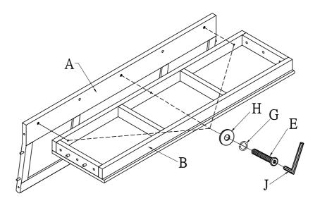
Tighten the Back Rest (A) Seat (B) Legs(C)(D) by Bolt (F) and Bolt(E)Lock Washer(G) Flat Washer(H)with Allen Wrench(J).
