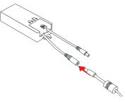
2. Ensure the power supply is unplugged from 120V power. Connect the male barrel plug from the power supply to the female INPUT barrel plug on the Doppler Motion Sensor.
