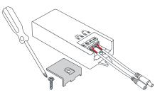
2. Use a #2 Phillips to loosen the screw and remove cover from Doppler Motion Sensor.
