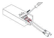
**3.** Use a flat blade screwdriver to loosen terminals for the Male Plug and Female Plug Connectors; remove from device.
