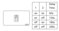
5. The small switches on the side of the Doppler Motion Sensor control how long the lights will stay on once motion is detected. Follow the diagram printed on the Sensor to select desired length of time.
