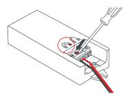
4. From the Power Supply, insert the end of one set of stripped wires into the INPUT terminals on the Sensor, Red wire to (+) and Black wire to (-); tighten screws.
