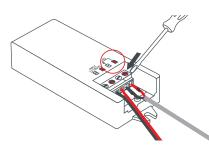
Insert the end of the stripped wires into the OUTPUT terminals on the Sensor, Red wire to (+) and Black wire to (-); tighten screws. Insert the other end of the wires into the LED lights.
