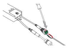
4. Loosen terminal screws on the Female Barrel Connector. Insert one end of the wire into the terminals, Red to (+), Black to (-); tighten screws. Connect the other end of the wire to the LED lights and plug Power Supply into power source.
