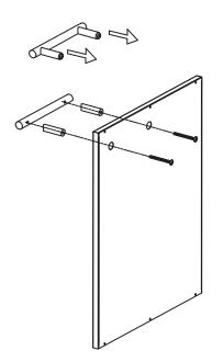
USING THE SCREWS PROVIDED, ATTACH THE DOOR HANDLES TO THE TWO PANTRY DOORS.
