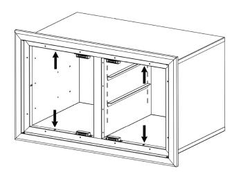
With the drawers and shelves removed, after the pantry has been inserted into the cut out, attach to the upper and lower sleepers using 4 screws in the locations shown.
