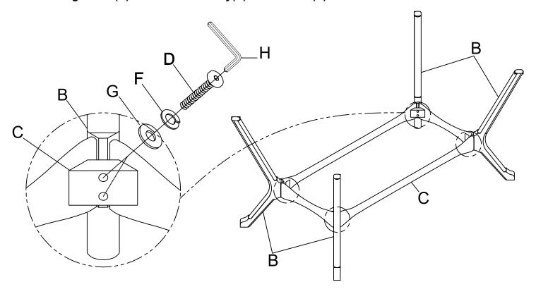
Attached Leg Frame(C) to the Table Top(A). Use Allen Bolt(E) Lock Washer(F) and Flat Washer(G) on holes of Table Top(A). Turn the Allen Key(H) in Allen Bolt(E).
