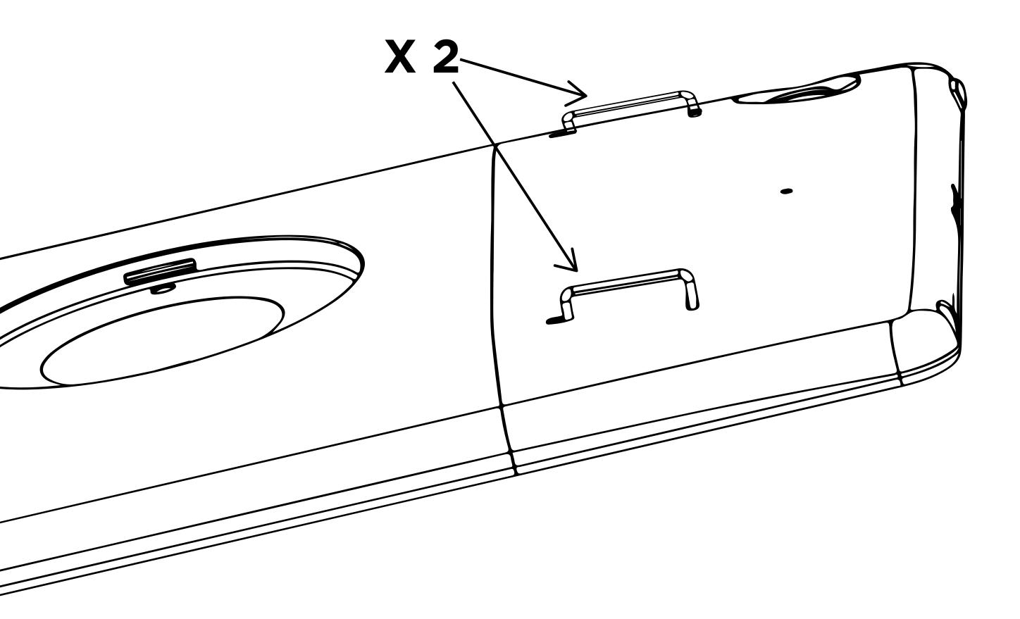
4. Insert the IPORT CONNECT Hand Strap under both strap loops with the Velcro facing out from the case, fold over the Hand Strap and attach to the Velcro. Adjust hand strap to a snug but comfortable fit around the top of your hand.
