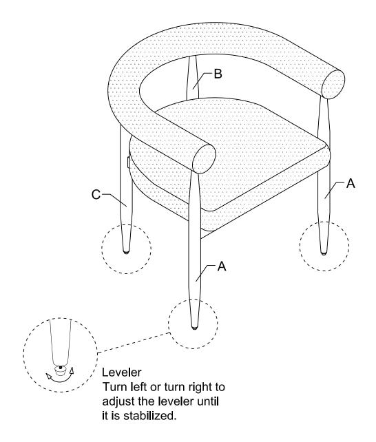
Stand the chair on an even surface and check for balance. If the chair wobbles slightly, apply downward pressure on the uneven leg and tighten the bolts to correct the imbalance. Once the chair is balanced, apply downward pressure evenly in the center of the chair and tighten all bolts, being careful not to over-tighten beyond the hole depth.
