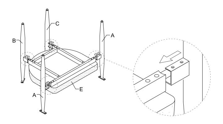
Attach the Front and Back Leg (A, B, C) to the Seat Cushion (E) using Bolt (F), Lock Washer (H) and Flat Washer (I) with the Allen Key (J).
