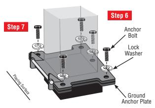
**Step 8:** Snug tighten the five anchor bolts, then check goal assembly with a level and inspect visually to determine if it is parallel and plumb to the playing surface.
