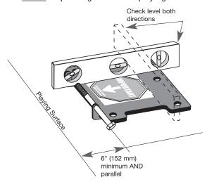
**Step 6:** Position 6" ground anchor (G2660) in center of hole with hinge side toward and parallel with playing surface. Using a level, ensure the anchor is level front-to-back and left-to-right. All edges of the ground anchor must be 6" (15.2 cm) away from all sides of hole and the top of the ground anchor within a range of 1"- 3" (25-75 mm) above the level of the playing surface.
