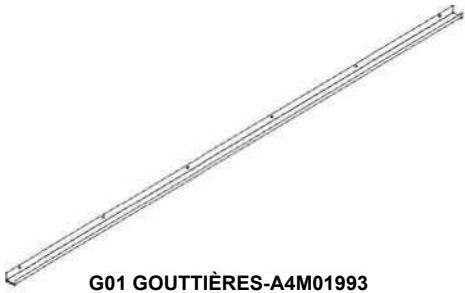
G01 GOUTTIÈRES-A4M01993 (x1) 1 9/16"x1 15/16"x108 7/8" (40x50x2765)
