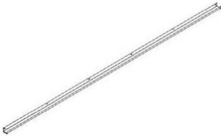
G03 GOUTTIÈRES - A4M04120 (x1) 1 9/16"x1 15/16"x111 11/16" (40x50x2837)
