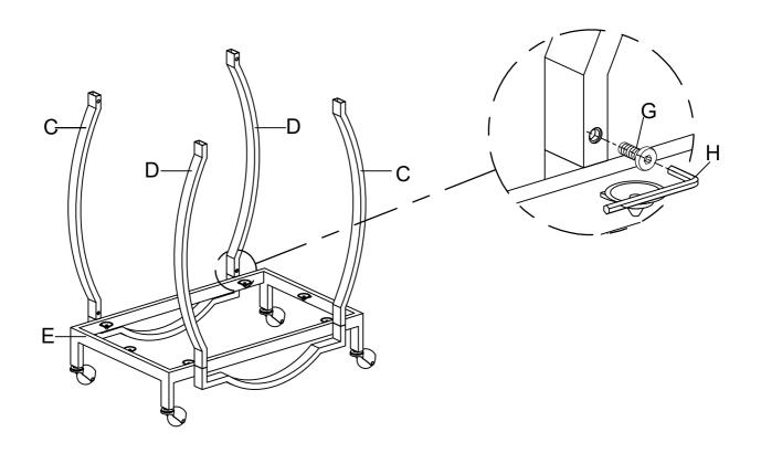
Attach Top Frame (B) to Stretcher (C) and Stretcher (D) using Bolt (G) by Allen Key (H) as below shown.
