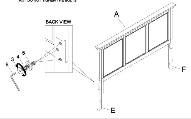
STEP 2 Assemble Headboard Crossbar (D) to HB legs (E) and (F) by using Allen Key (4) with hardware 2, 4, and 5.
