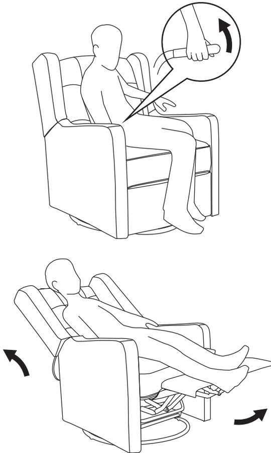
The chair can be made to recline by simply pulling the arm located at the inside right of the base (B) and pressing the back against the backrest.
