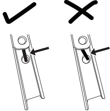
Make sure the locking mechanism on each metal glide is aligned in the **center**.
