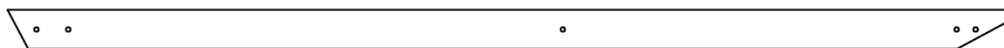
E51 | CALE ANGULAIRE - W4L16004 (x2) | 1 \frac{7}{16} po x 3 \frac{3}{8} po x 87 \frac{3}{16} po (36 x 86 x 2214)
