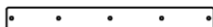
O01 | SUPPORT MURAL - W4L16081 (x2) | 5/8 po x 1 3/8 po x 13 po (16 x 34 x 330)
