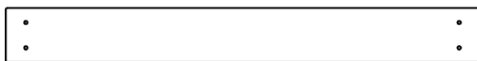
M24 | PANNEAU MURAL - W4L16061 (x9) 5/8 po x 3 3/8 po x 29 5/8 po (16 x 86 x 752)
