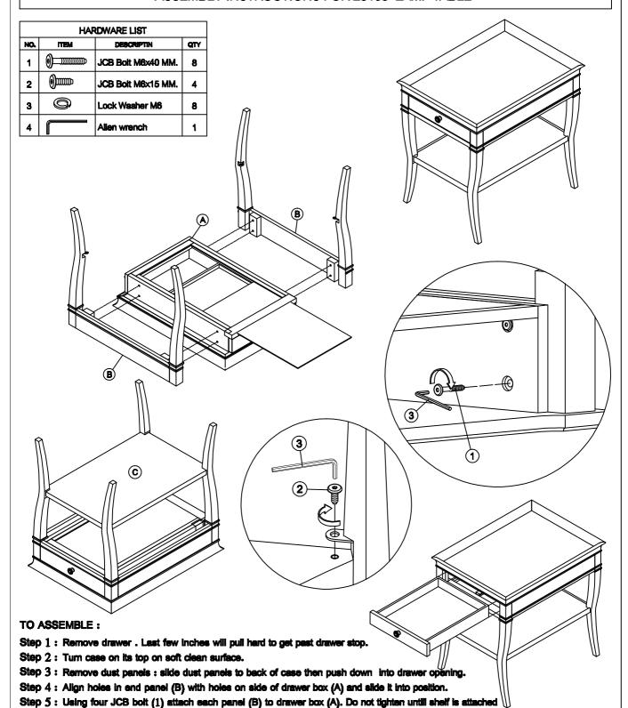
Step 6: Attach the shelf (C) to legs (B) in the notch, tighten using JCB bolt M6x15 (2) with allen wrench (3).
