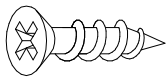
30 x 88 M3.5 x 12mm Screw M3.5 x 12mm de la vis M3.5 x 12mm el tornillo
