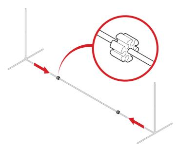
Locate the sleeves on the part B net and slide it over the top net supports.
