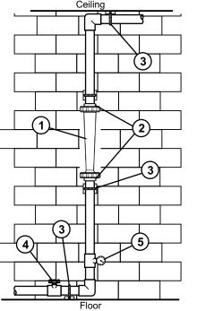
tools. Union nuts should be hand tightened only. DO NOT OVER-TIGHTEN!
